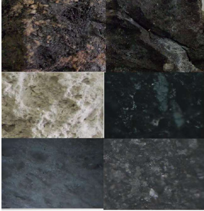
Figure 1. The macro and micro images of Boiler slag, volcanic slag, Tatvan Pumice.
