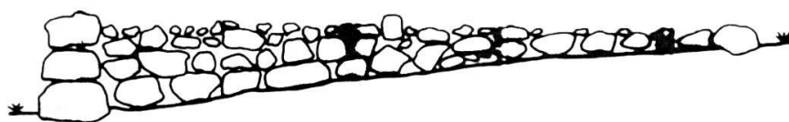
Fig. 3. Technique for Low Pitched Terrains (French, 1981)
